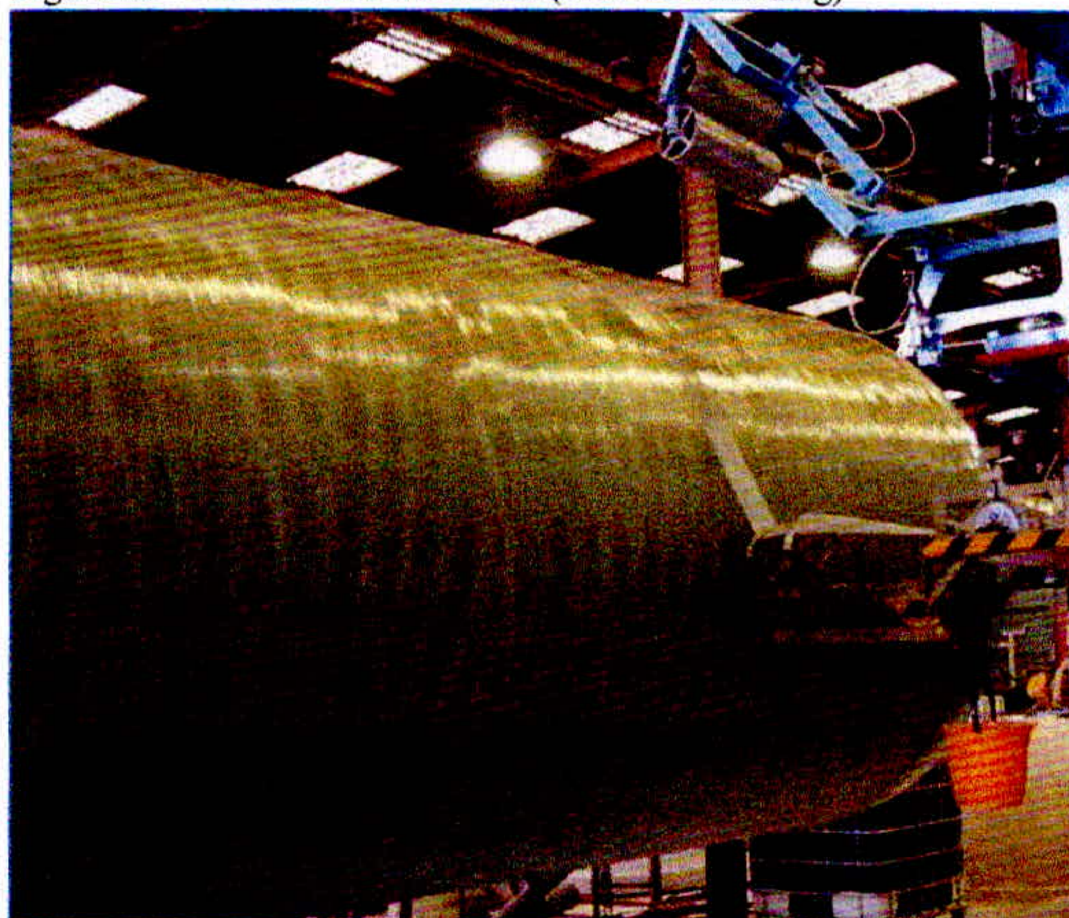
Figura 10 – Enrolamento helicoidal (Filament Winding)
