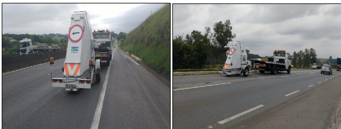
Figura 5 e 6 – FWD(Falling Weight Deflectometer)
