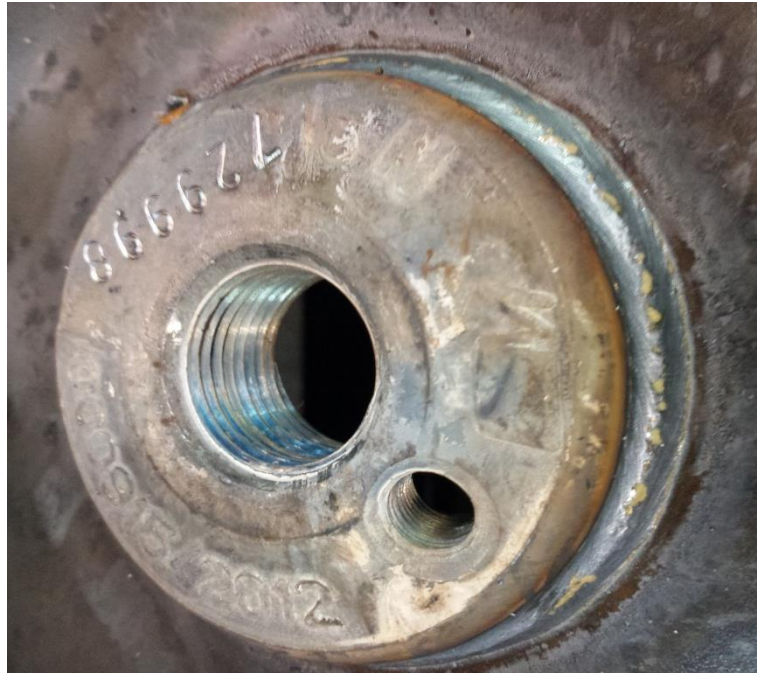
Figura 25: Solda com arame Metal Cored
